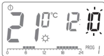
4. In the top left corner a blinking day symbol will appear. Turn the knob clockwise or counter clockwise to set the day desired and confirm with the
